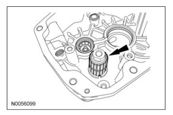
6. Remove the reverse idler gear shaft.
