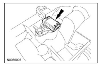
2. Remove the reverse lockout solenoid bolt and the reverse lockout solenoid.
